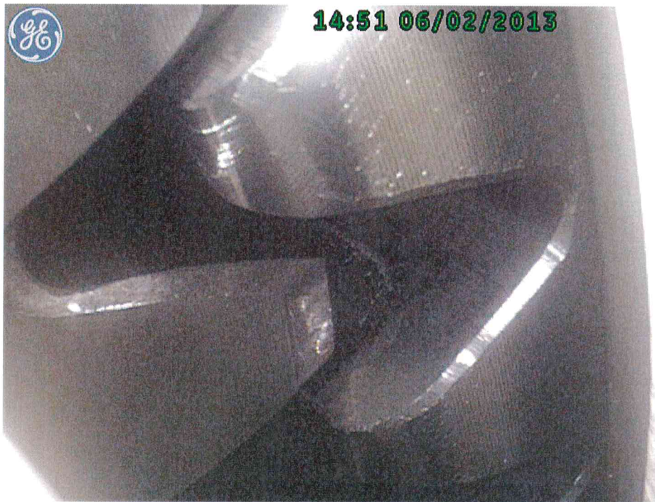
Picture 1: Intermediate gear mesh, planet- ring gear
